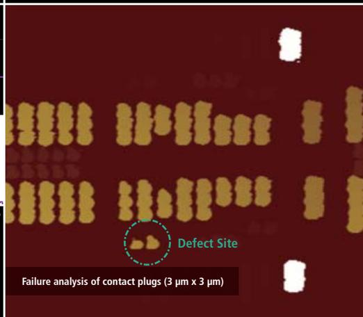
Failure analysis of contact plugs (3 μm x 3 μm)
