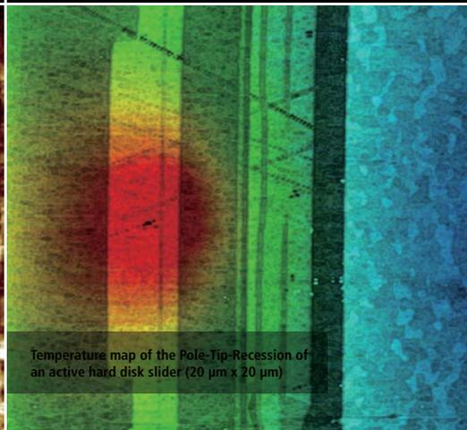
Temperature map of the Pole-Tip-Recession of an active hard disk slider (20 μm x 20 μm)
