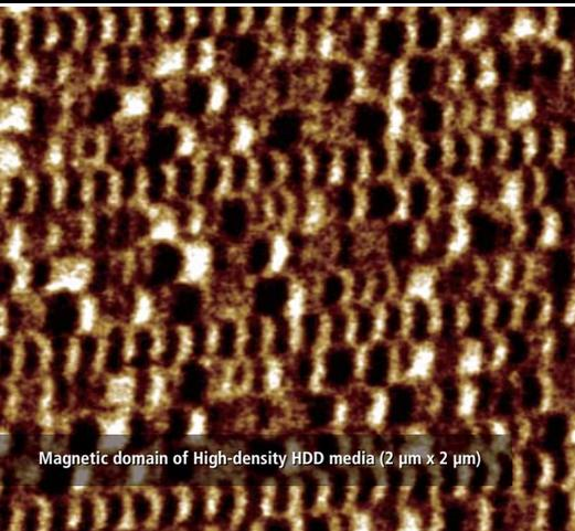
Magnetic domain of High-density HDD media (2 μm x 2 μm)
